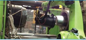
Large Part Injection Molding with Robotic Removal & Assembly
