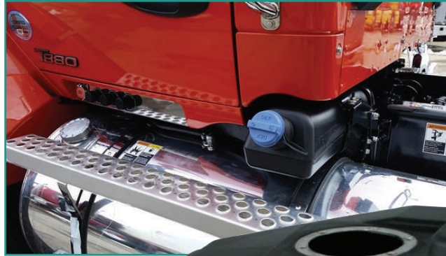
Over-molded neck feature on PACCAR DEF Tank
